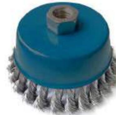
Wire brush plait straight with thread. Suitable for removing rust, paint and cleaning metal surfaces. Twisted wire for excellent durability on harder surfaces and longer life. Suitable for use on all wheels with M14 thread.
